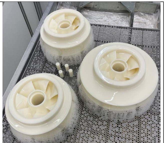
Three impellers on a print platform before post-processing (source: KSB)
