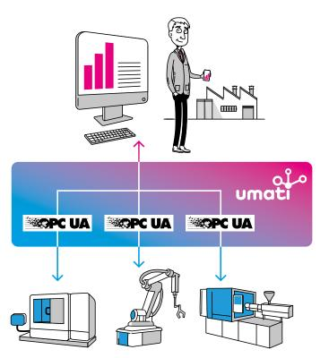
How umati works: several machines with OPC UA servers using Companion Specifications endorsed by umati, implemented according to umati guidelines, are connected to one IT system with an OPC UA client.
