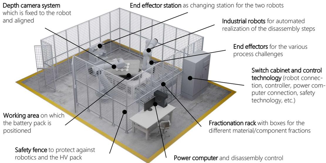
Concept illustration of a prototype cell from the DemoSens research project
