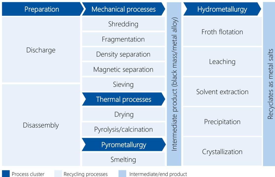
The recycling processes listed here can be combined with each other in different ways in recycling routes. Not all recycling processes have to be used.
